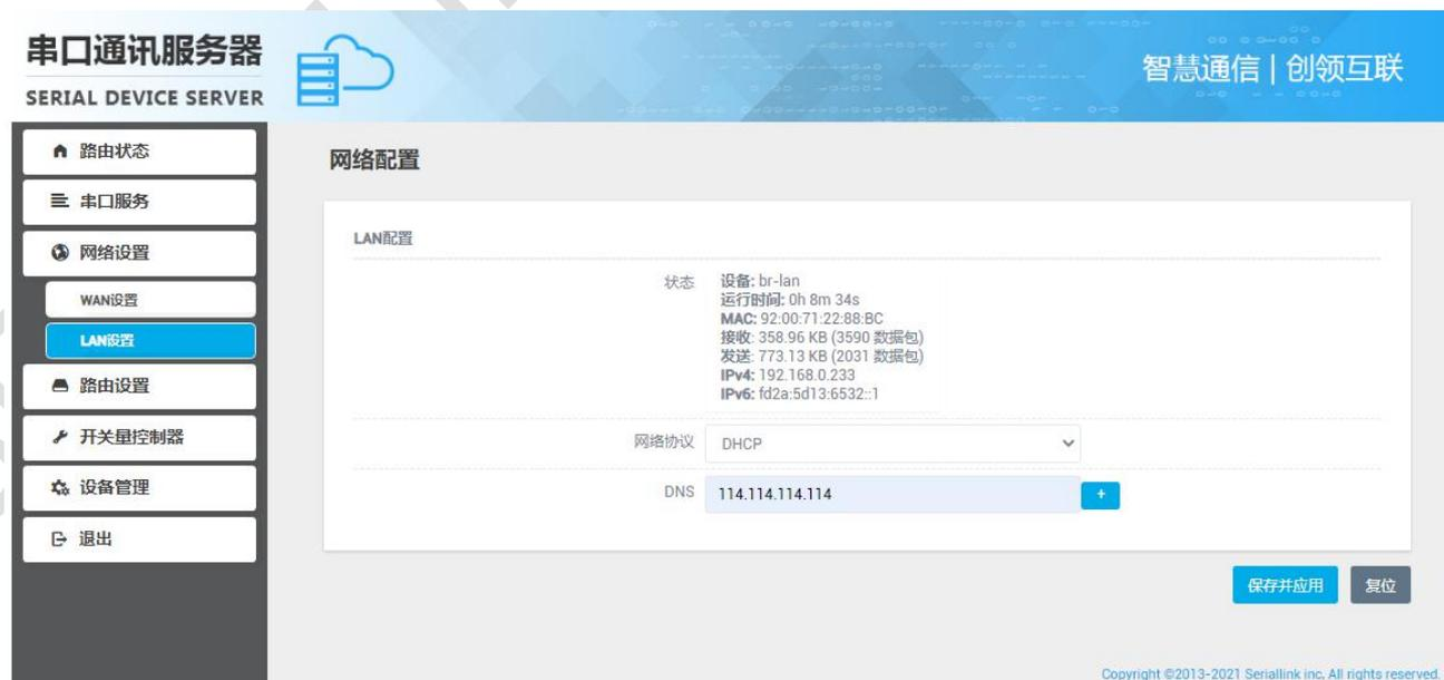
The screenshot shows the 'LAN配置' (LAN Configuration) page in the Serial Device Server web interface. The network protocol is set to 'DHCP'. The DNS field contains the value '114.114.114.114'. The status section shows device information for 'br-lan'.
