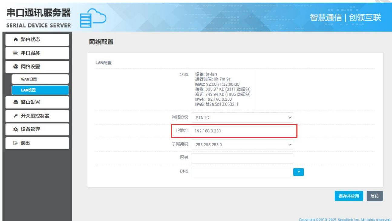
The screenshot shows the 'LAN配置' (LAN Configuration) page in the Serial Device Server web interface. The network protocol is set to 'STATIC'. The IP address field is highlighted with a red box and contains the value '192.168.0.233'. Other fields include '子网掩码' (Subnet Mask) set to '255.255.255.0', and 'DNS' with a plus sign to add more addresses. The status section shows device information for 'br-lan'.
